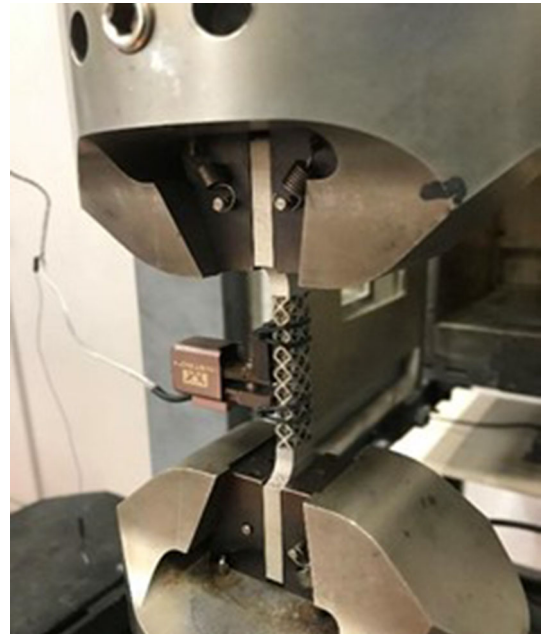
Fig. 3. Experimental setup of the uniaxial tensile test
