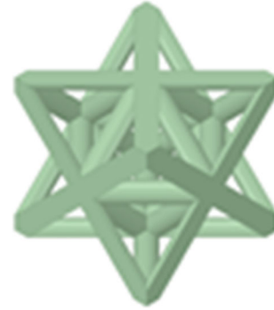
Fig. 2. CAD model of the Octet-truss cellular structure
