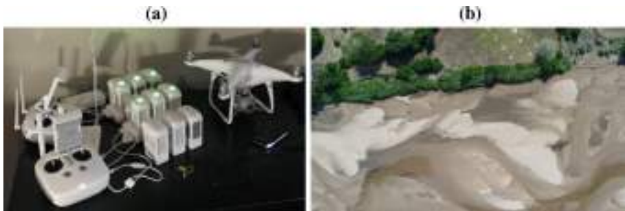
Fig. 3 a DJI Phantom 4 Pro, remote controllers and set of 9 batteries with charging hubs; b example of picture taken from the on-board camera of the DJI Phantom 4Pro
