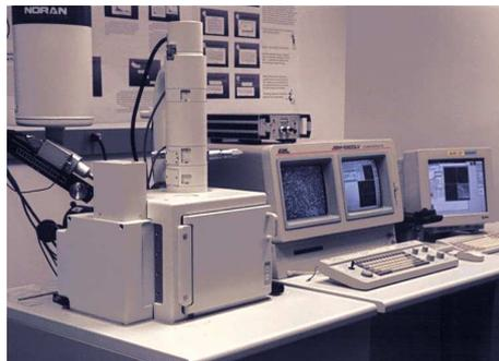
**Fig. 3.4:** Scanning Electron Microscope (SEM): a typical SEM instrument, showing the electron column, sample chamber, electronics console, and visual display monitors.
