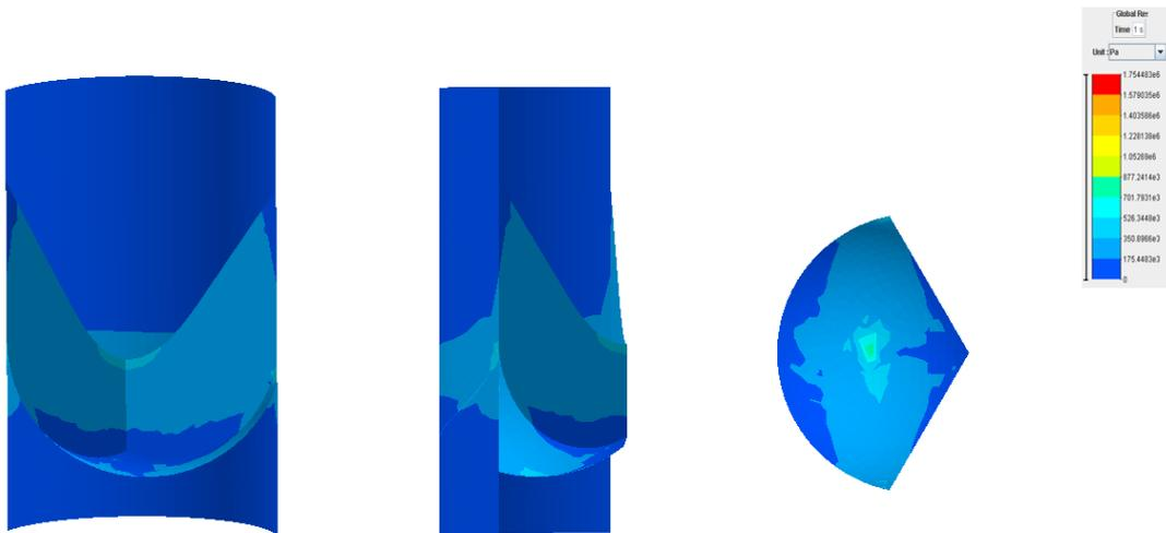
Figure 4.30: Equivalent stresses of the valve after diastole load condition. In order a frontal, tridimensional and top view.
