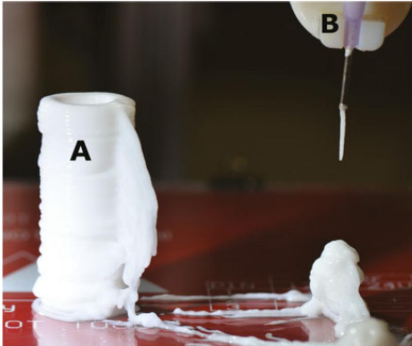
Fig. 1. Completed actuator print on the heated bed after print completion (A). Also shown is the printer's extruder (B).
