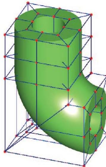
Figure 2.44 The control lattice for the pipe.
