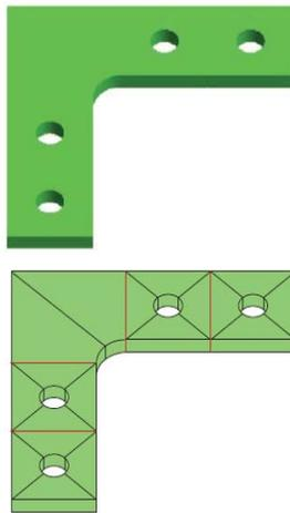
Figure 2.29 The bracket on the top is exactly and concisely represented by five simple NURBS patch (patch boundaries are shown in red, element boundaries in black). The patches match geometrically as parametrically on the internal faces where they meet.
