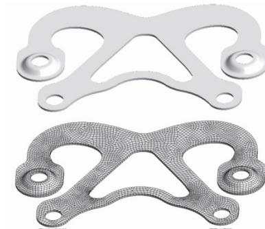
mechanical spring for a chiseling tool
