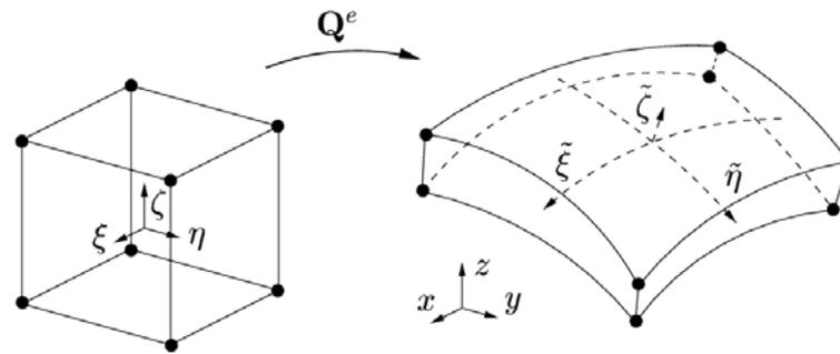
$Q^e$  is a mapping describing the **true** geometry i.e. B-splines, NURBS...
