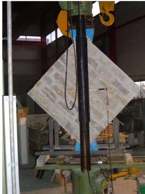
Figure 1.10: Diagonal compression setup
