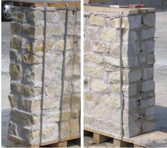
Figure 1.5: Wall edge before cut (left) and after cut (right)
