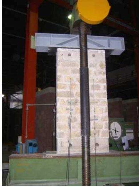
Figure 1.6: Vertical compression test setup
