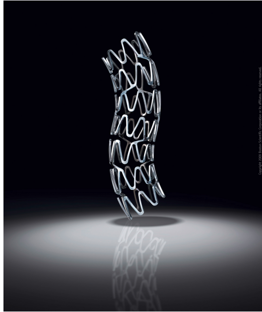
Figure 2.4: Element stent from Boston Scientific Corp. Balloon expandable open cell sequential ring design with periodic peak to peak non flex connections.
