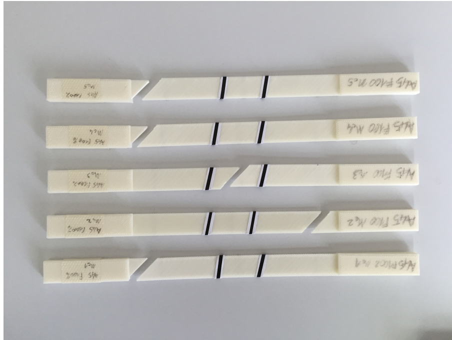
Figure 11.4: 45 Degrees Fibers Specimens Failure Point
