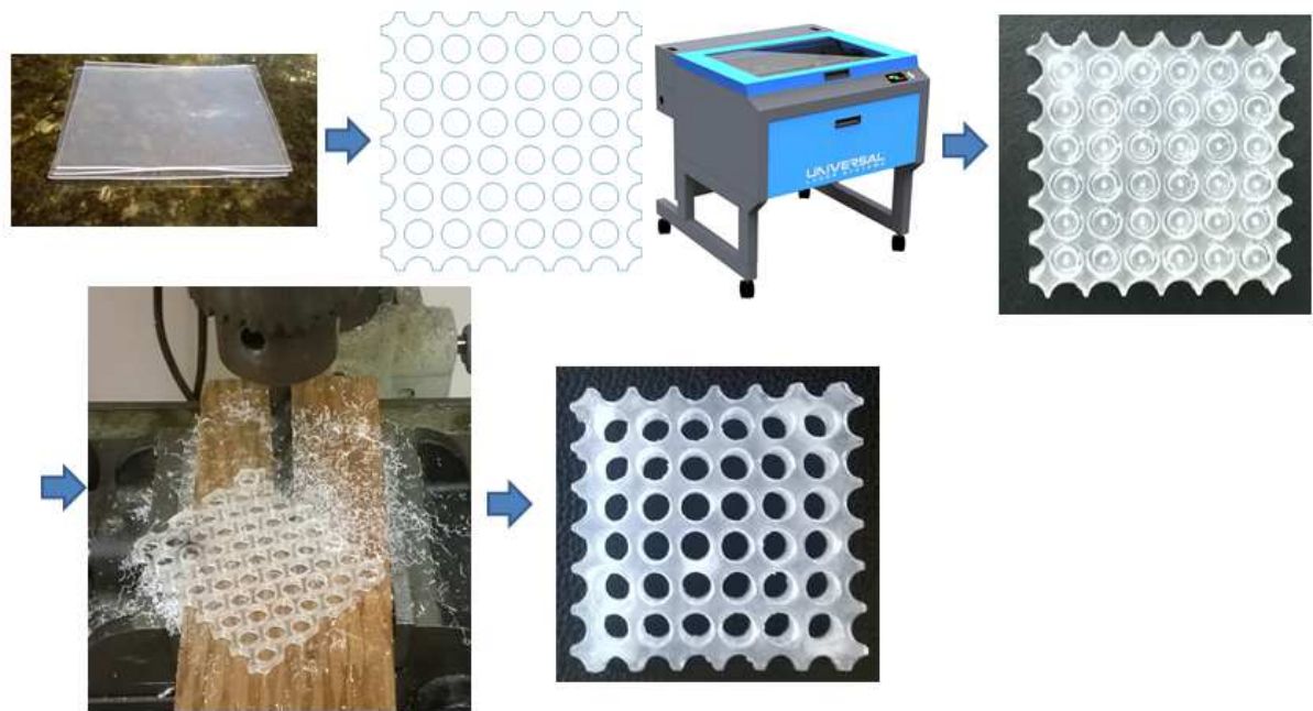
Figure A.6: Manufacturing procedure: the layers are overlapped and heated in order to glue them; the external shape and the holes locations are then obtained through a laser-cutter; finally, the holes are drilled.
