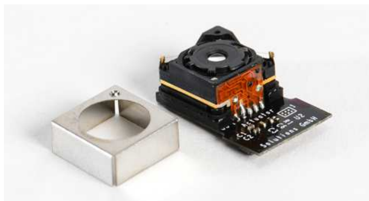
Figure 1.7: SMA-actuated autofocus for a miniature camera by Actuator Solutions GmbH [38].
