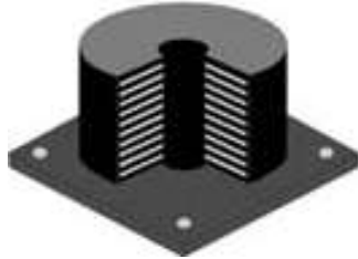
Figure 2.4. Laminated rubber bearing structure [from Dolce et al. [2007a]]
