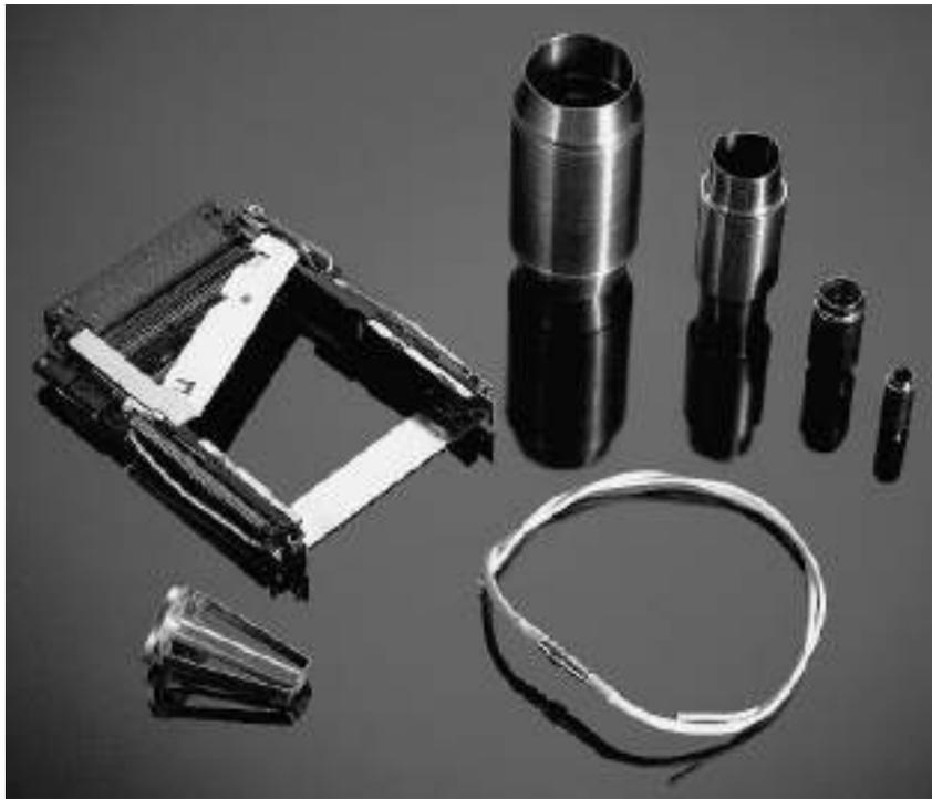
Figure 1.17: Shape memory devices. Clockwise from top left: memory card ejector mechanism for laptop computers; Cryofit<sup>®</sup> hydraulic pipe couplings; Cryocon<sup>®</sup> electrical connector; fire safety lid release for public garbage receptacles (Schwartz, 2002).
