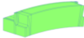
Figure 3.50. NASA ATC. Typical 15° segment of an end rib. Mesh 1 (coarsest mesh).
