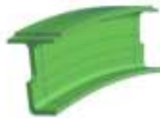
Figure 3.45. NASA ATC. Typical 15° segment of the main rib. Mesh 1, the coarsest mesh, encapsulates the exact geometry.
