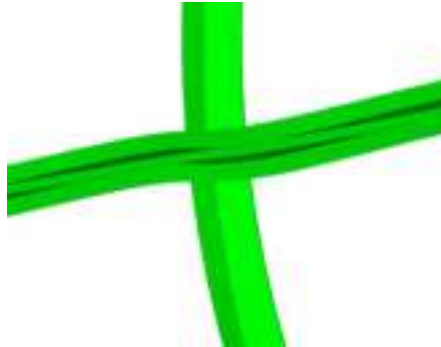
Figure 3.64. NASA ATC. Detail of first torsional mode for the frame assembly; stringer-main rib junction.
