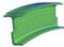
Figure 3.47. NASA ATC. Typical 15^\circ segment of the main rib. Mesh 3. Further refinement may be necessary to resolve the solution, as is the case with standard finite element analysis, but the geometry is never altered as the mesh is refined.
