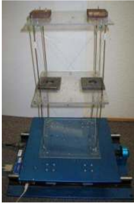
Figure 6.1. Elevation view of the reduced-scale frame mounted on the shake table.
