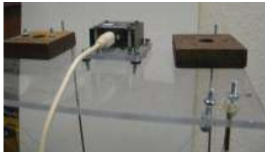
Figure 6.2. Close-up view of the top floor. Note the accelerometer, the steel masses and the connection between the plexi-glass sheet and the wire.
