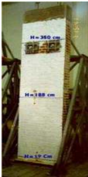
Figure 3.6. Masonry wall tested by Castellano [2000] and Indirli et al. [2000] (left) and wall connection with superelastic SMA devices (right).
