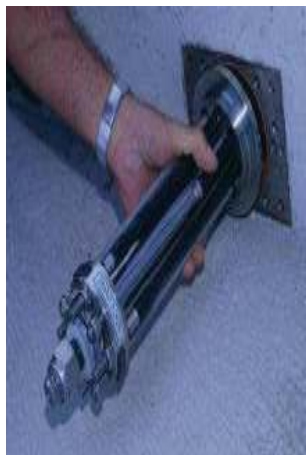
Figure 3.10. Particular of the SMA device utilized for the seismic upgrading of the Basilica of St Francis in Assisi, Italy.
