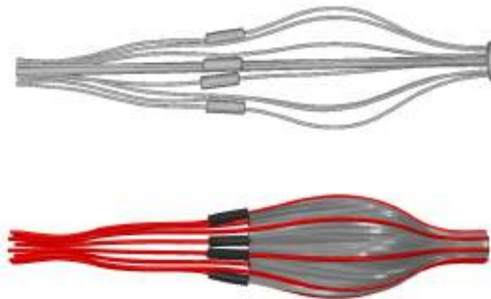
**Figure 2.6:** Partially deployed filter: micro-CT image (top panel); numerical simulation (bottom panel).
