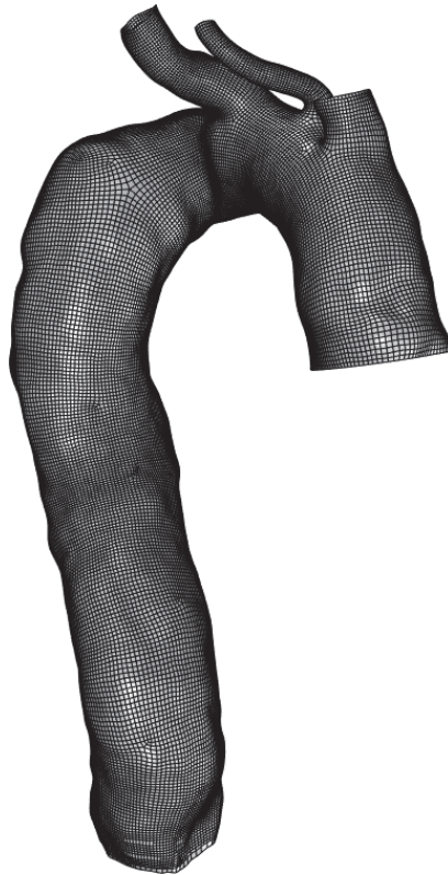
Figure C.1 Example of bicubic T-mesh created in Rhino and imported in FEAP.
