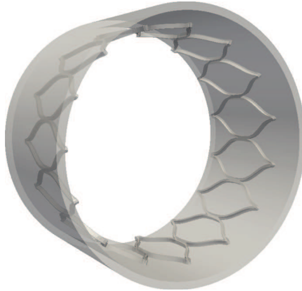
Figure 6.5 Stent model in undeformed configuration with its cylindrical crimper.
