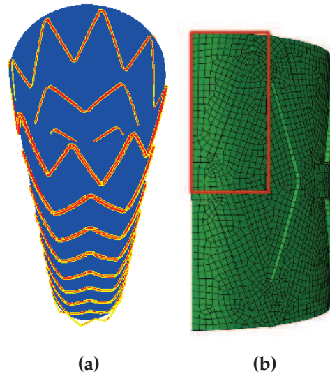
Figure 7.10 (a) Example of application of the "aba2feap" command. The Medtronic Valiant stent (46-46-150 mm) was first created in Abaqus and then imported in FEAP for testing the conversion code. (b) Quarter of cell of the same stent-graft mesh used for obtaining the properties of the RVE to employ in the simulations.
