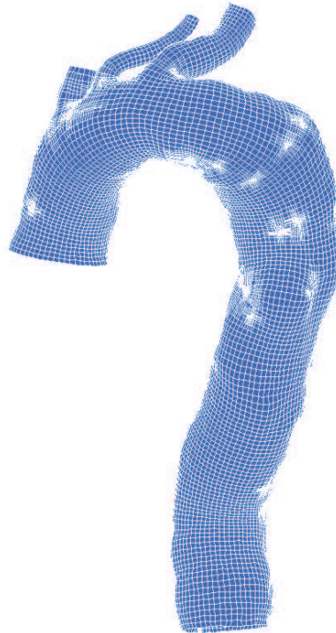
Figure 5.13 Fine mesh location around extraordinary points in IgA-FEAP for the patient-specific model depicted in Figure 5.11a.
